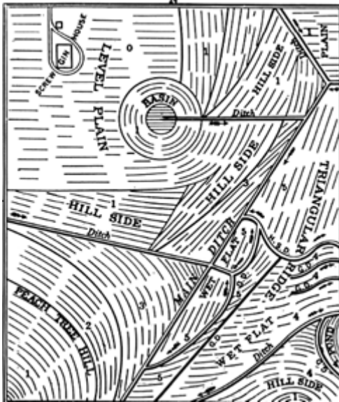
Figure 7.--Sorsby's plan for diversified erosion control on a 45 acre plot: 0, Straight rows run by the eye; 1, level culture; 2, level culture with guard drains; 3, grading method No. 1; 4, grading method No. 2; 5, grading method No. 3.
